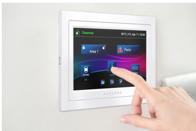
TM70 installed with in-wall optional bracket
