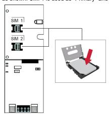
one SIM card is used, insert into SIM 1.
