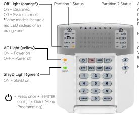
Arm (red), Sleep (yel), Stay (grn) On = Partition armed Off = Partition disarmed Flash = Exit Delay Fast Flash\*= Exit Delay (final 10 sec.) Fast Flash\*= Partition in alarm
